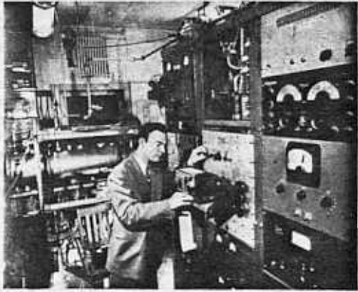
The first atomic-beam clock, developed at the National Bureau of Standards in 1950-52. It used a line in the hyperfine-structure spectrum of cesium. (NBS photo.)
