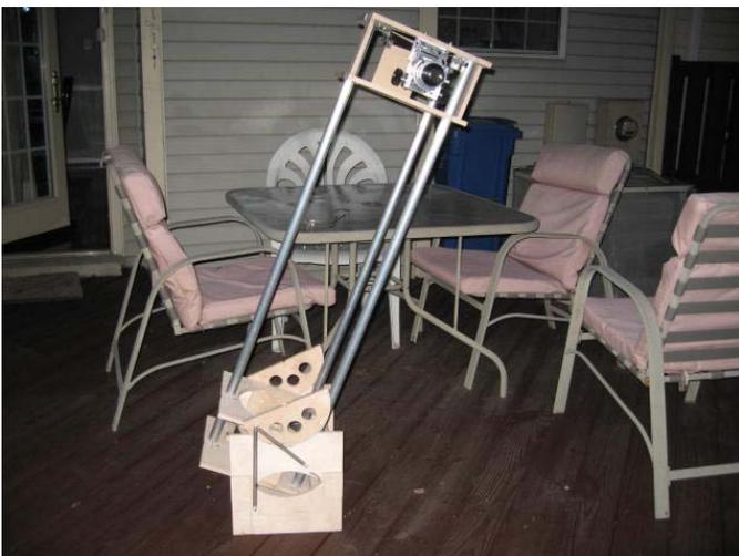
Last month we profiled a Crayford focuser built by Prasad Agrahar, a student at the NCA Amateur Telescope Making class. Here is Prasad's focuser again, during first light on his assembled 8 inch Dobsonian-mounted Newtonian reflecting telescope.
