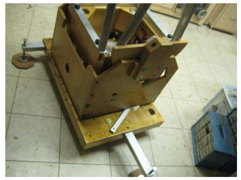
The telescope is a rugged truss-tube design, with adjustable feet on the legs extending from its rocker box. The legs give the telescope additional stability, and the adjustable feet help keep it level on uneven ground. A small round bubble level permanently mounted on the base is helpful for setting up the telescope evenly. In the photo below, the primary mirror's cell and cooling fans are visible at the bottom of the telescope's rocker box.
